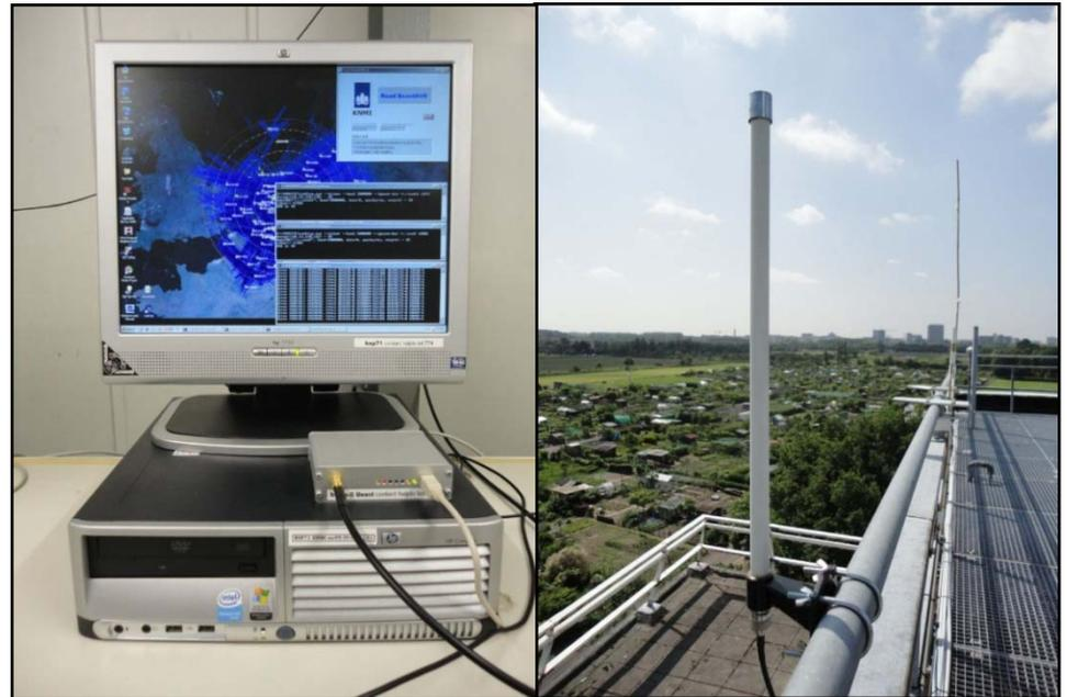
Data acquisition PC and Mode-S Beast (left) and GP1090 antenna on the roof of the KNMI premises (right).
