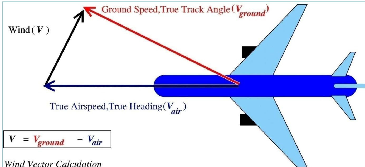
Schematic representation of wind derivation from aircraft flight information. The wind vector (black) is deduced from the difference between the ground track vector (red) and the orientation (heading) and speed of the aircraft relative to the air (dark blue). The ground track vector is constructed by ground speed and true track angle. Note that both heading and ground track angle are defined with respect to true north.
